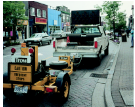
Figure 13. A falling weight deflectometer was used to evaluate the structural capacity and remaining life of the pavement.
