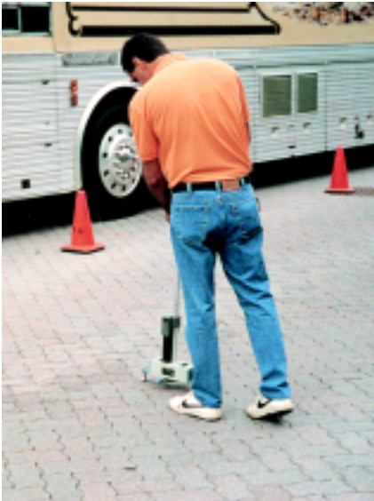
Figure 12. Rut depth measurements after eight years of traffic showed rutting to be slight.
